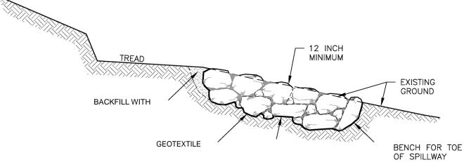
Figure 20: Rock Retention Wall
