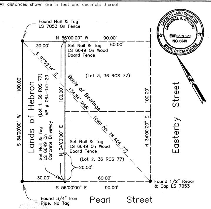
Basis of Bearings being the calculated line between found monuments as shown on 36 ROS 77, M.C.R. Bearing of S 07\*59'14" E
