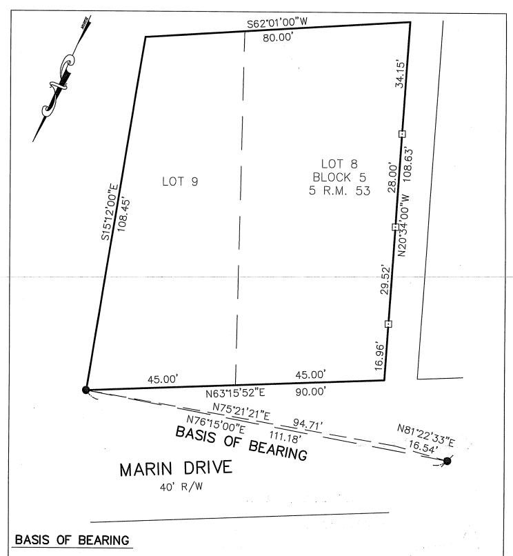
THE BASIS OF BEARING FOR THIS SURVEY IS N76°14'59"E BETWEEN FOUND POINTS PER 12 O.S. 73
