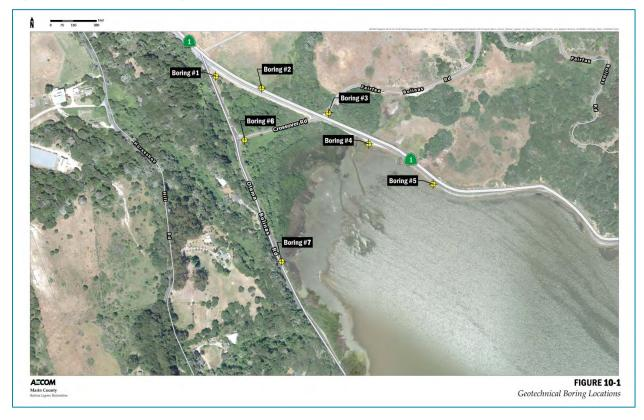
The groundwater levels as measured in the borings were approximately 1.5 feet to 10 bgs corresponding to an elevation range of 5 to 19 feet (NAVD 88). Initial readings were collected from wells B-1, B-2, B-4, and B-6; the water levels as measured are included in Table 1.
