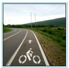
Figure 7. Class II Bikeway with Striped Lane for One-Way Bike Travel<sup>5</sup>
