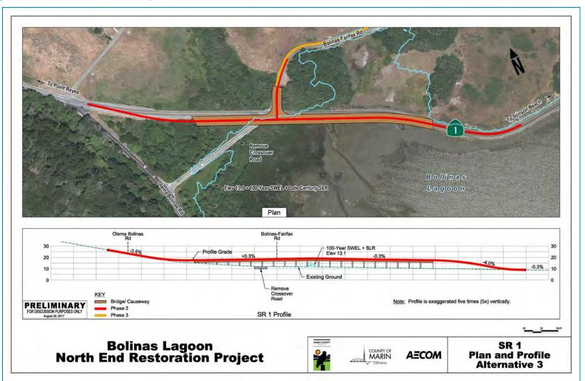
Figure 26. Alternative 3 – SR 1 Causeway Plan and Profile
