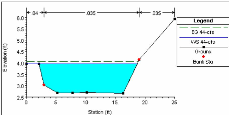
Figure 6. Cross-section at Station 897.11 (looking upstream) with a Bank-Full Capacity of 44-cfs Simulated in HEC-RAS
