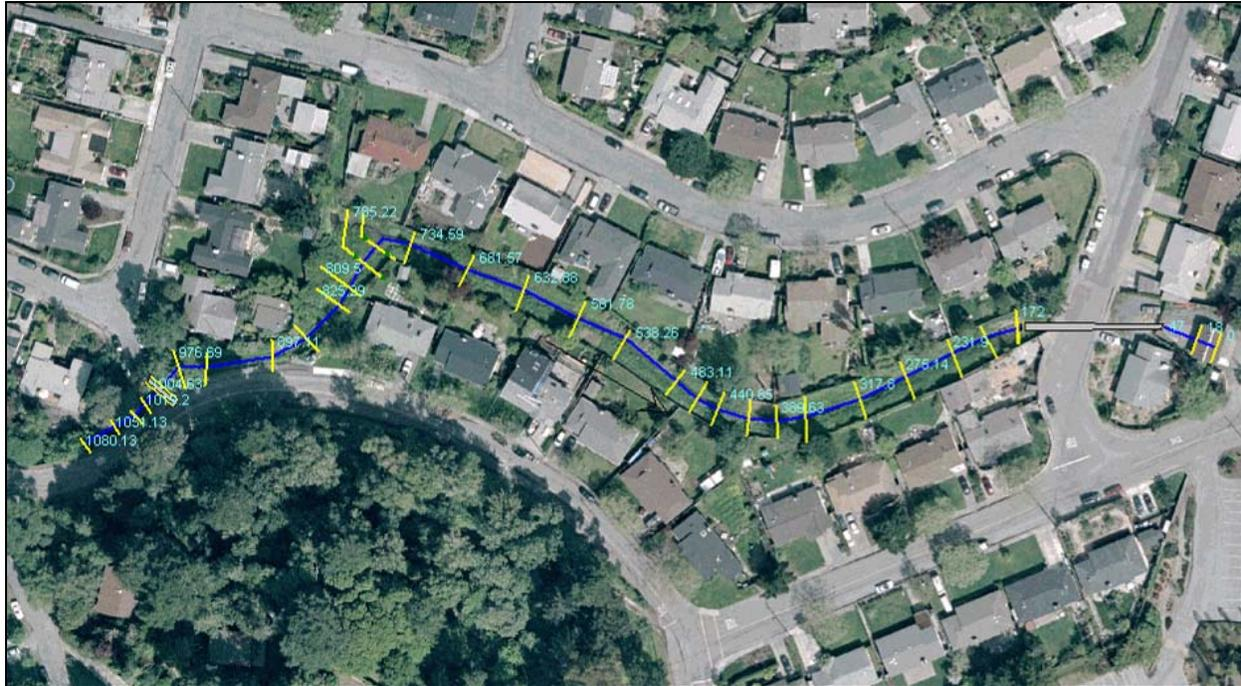
**Figure 4. Plan View of HEC-RAS Model and Cross-sections**
