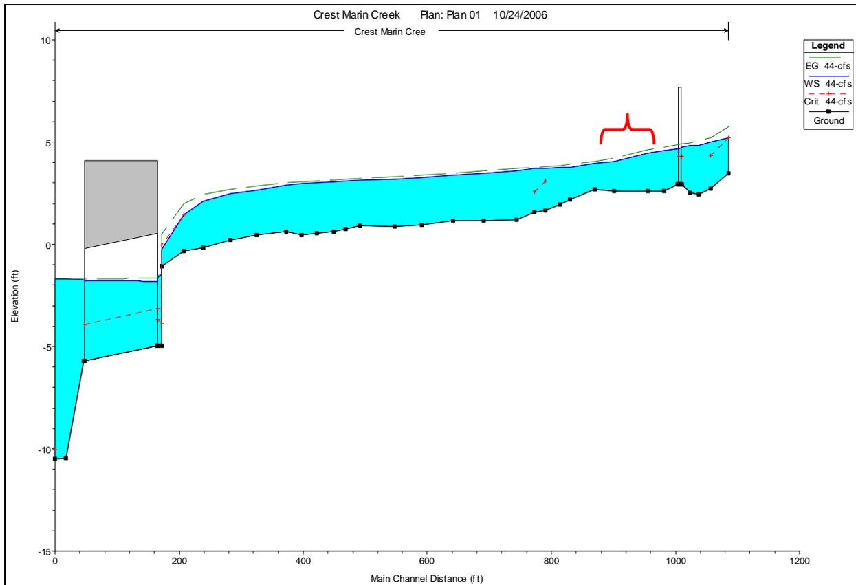
**Figure 9. HEC-RAS Profile of Crest Marin Creek Lower Reach at 44-cfs (Maximum channel capacity reached from station 809.5 through 976.69. Water surface elevation in pump station vault set at -1.71 feet (NGVD) corresponding with the high-level cut-off for Pump #1)**
