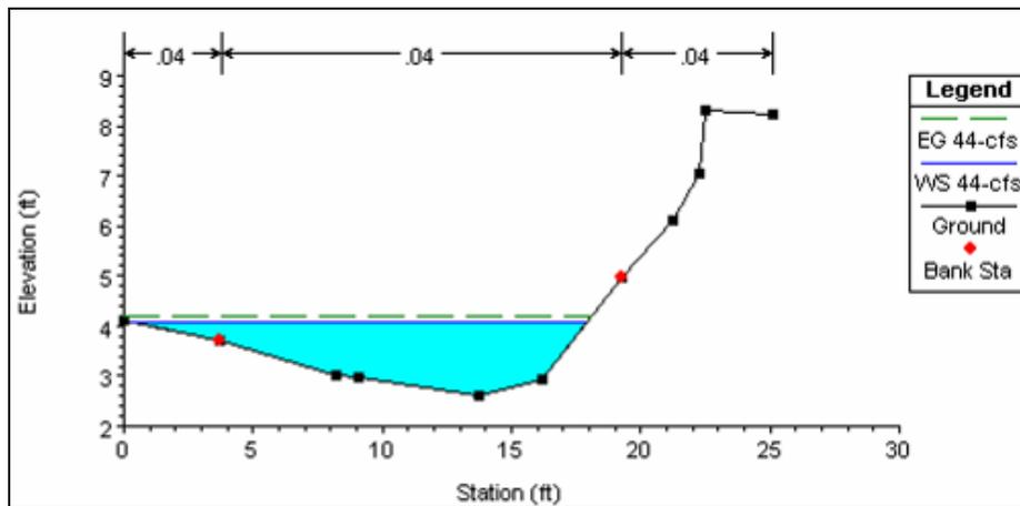
Figure 8. Cross-section at Station 897.11 (looking downstream) with a Bank-Full Capacity of 44-cfs Simulated in HEC-RAS
