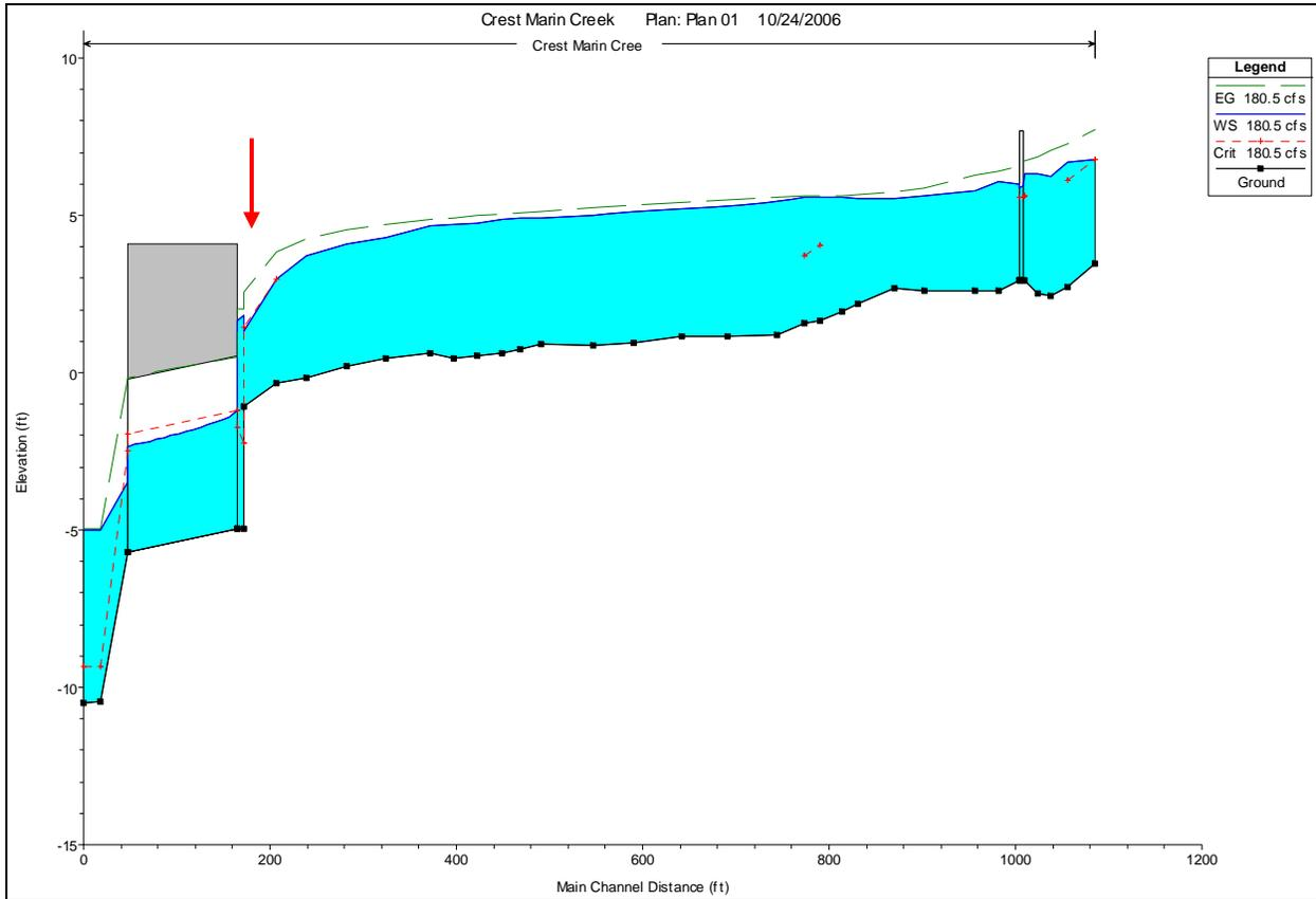
**Figure 12. HEC-RAS Profile of Crest Marin Creek Modeled Reach at 180.5-cfs (Water surface elevation in the pump station vault set at -5.0 feet (NGVD) corresponding with a normal low water elevation in the pump station)**
