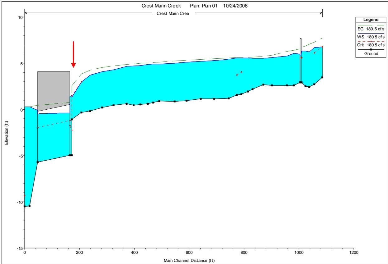
**Figure 10. HEC-RAS Profile of Crest Marin Creek Lower Reach at 180.5-cfs (Water surface elevation in the pump station vault set at 0.29 feet (NGVD) corresponding with a normal high-water elevation in the pump station, and all four pumps running simultaneously)**
