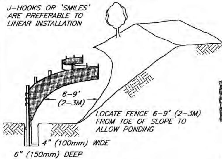
LOCATE FENCE 6-9' (2-3M) FROM TOE OF SLOPE TO ALLOW PONDING
