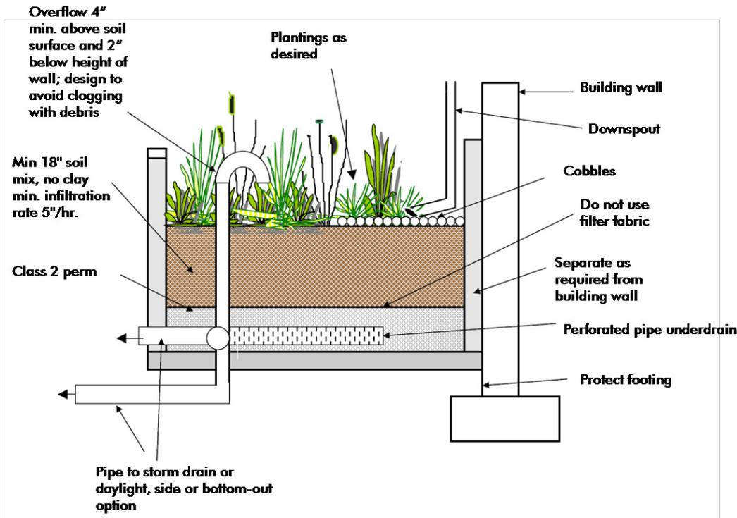
Planter boxes can be constructed adjacent to buildings or set into slopes. They are most effective when open-bottomed, but can also be built to eliminate seepage to native soils if necessary to protect foundations or slopes.
