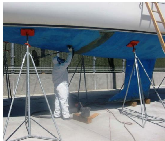
Contain blasting and sanding activities by using a vacuum sander with dust containment bags to prevent abrasives, dust and paint chips from entering stormwater.
