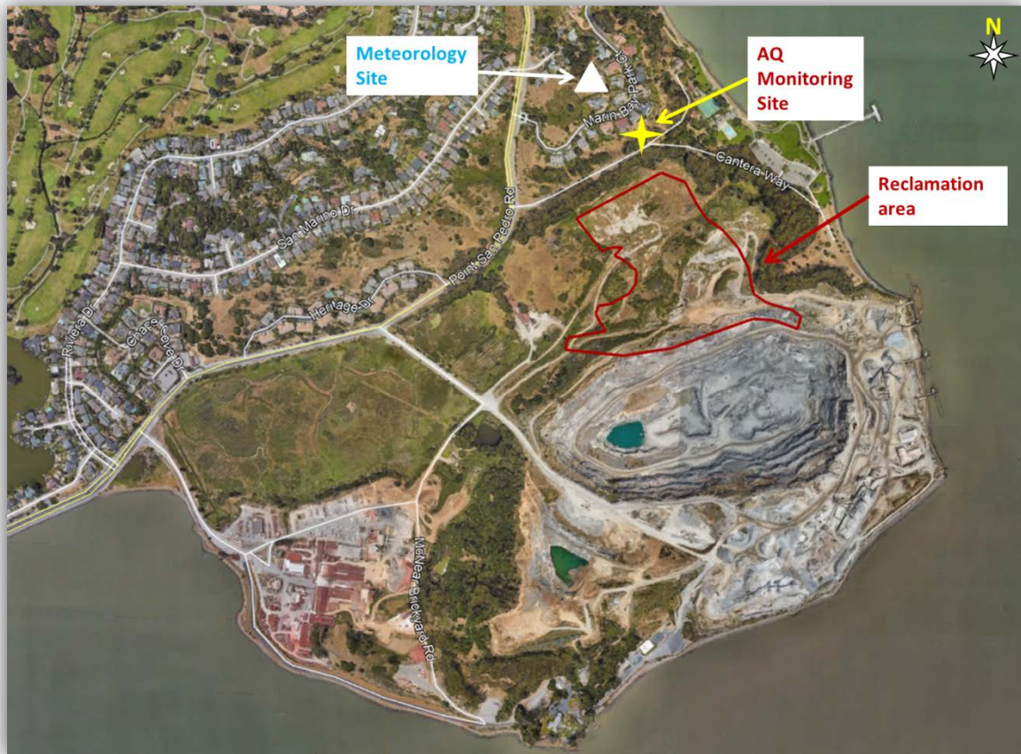
Figure 1. The San Rafael Rock Quarry and surrounding area. Monitoring sites for air quality (yellow cross) and meteorology (white triangle) data are north of the quarry. The northeast quadrant, where Reclamation Phase 1 will take place, is outlined in red.
