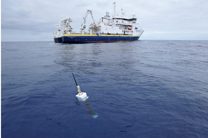
*One of the Argo array's buoys begins collecting ocean temperature data after a science team deploys it in the Atlantic Ocean. Credit: Argo / University of California, San Diego.*
