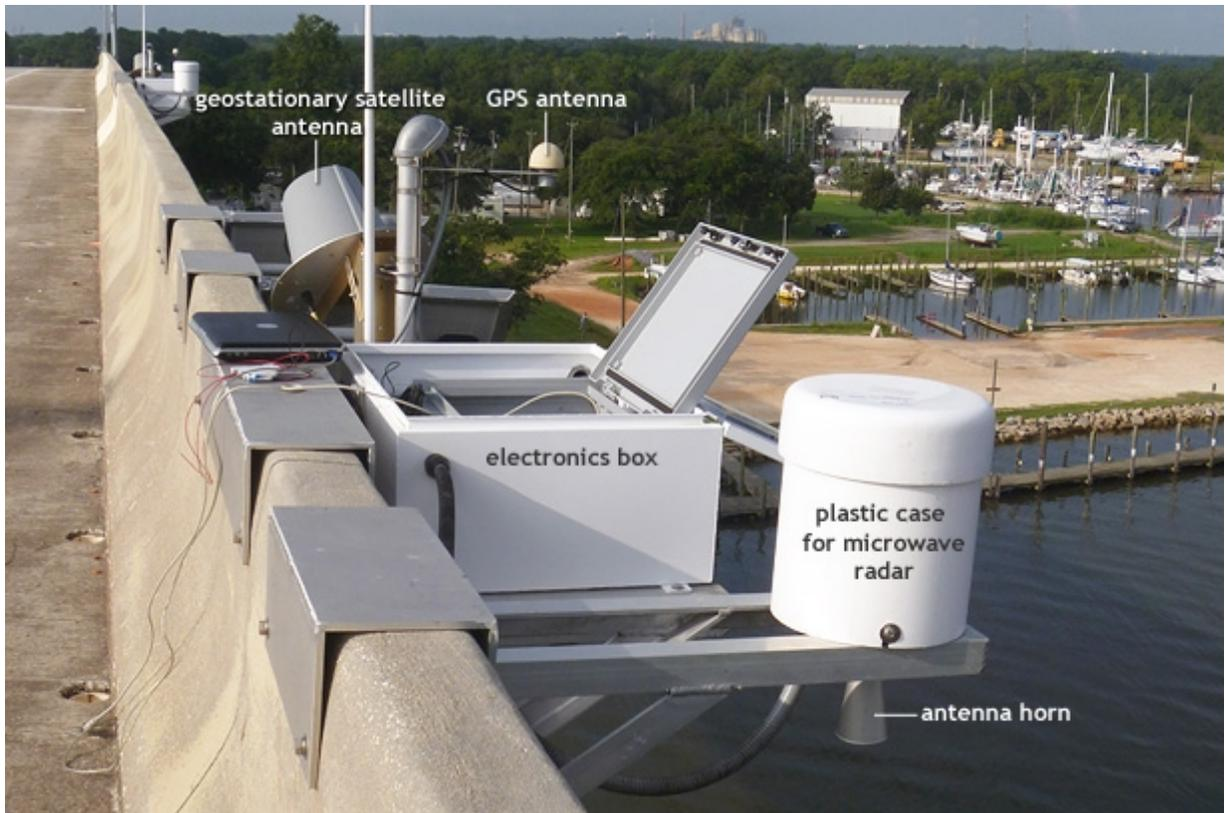
*A microwave radar attached to a bridge over the Dog River in Alabama. The radar, encased in the white plastic housing in the foreground, sends a pulse of microwave energy down toward the water surface and listens for the echo. The higher the water, the quicker return echo. NOAA photo courtesy Morgan McHugh.*
