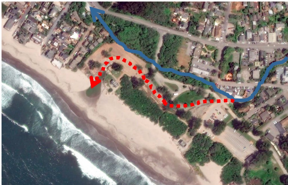
Figure 17 Easkoot Creek scour at NPS reach. Blue line shows channelized Easkoot Creek. Dashed red line shows flood flow avulsion through parking lots and dunes to beach
