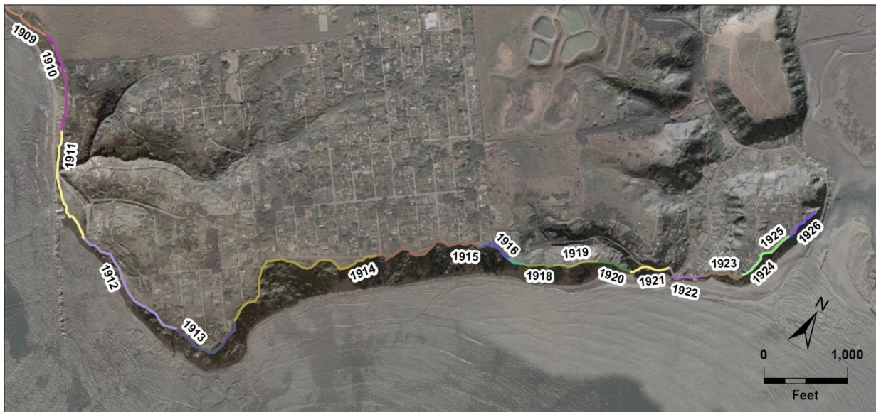
Figure 11. Bolinas 2010 bluff edge segmented by Pacific Institute (PWA 2009) study blocks.
