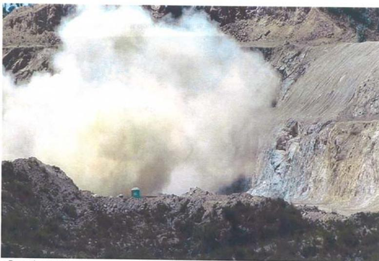
Promptly at 11:30 AM an explosion using 11,924 pounds of explosive was detonated on the northeast face of South Hill. A large dust cloud is observed rising into the atmosphere. The detonation moved 28,611 tons of rock with 22 holes shot. Note the green "porta potty" for scale.
