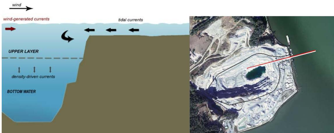
**Figure 4-1. Conceptual diagram of potential water exchange mechanisms in the proposed marina basin (left, not to scale) and cross-section location (right).**
