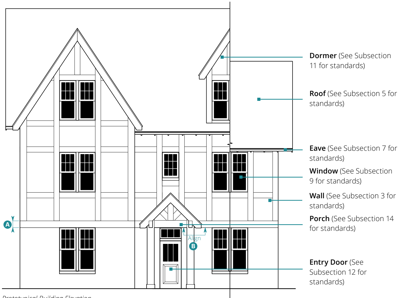
Prototypical Building Elevation
