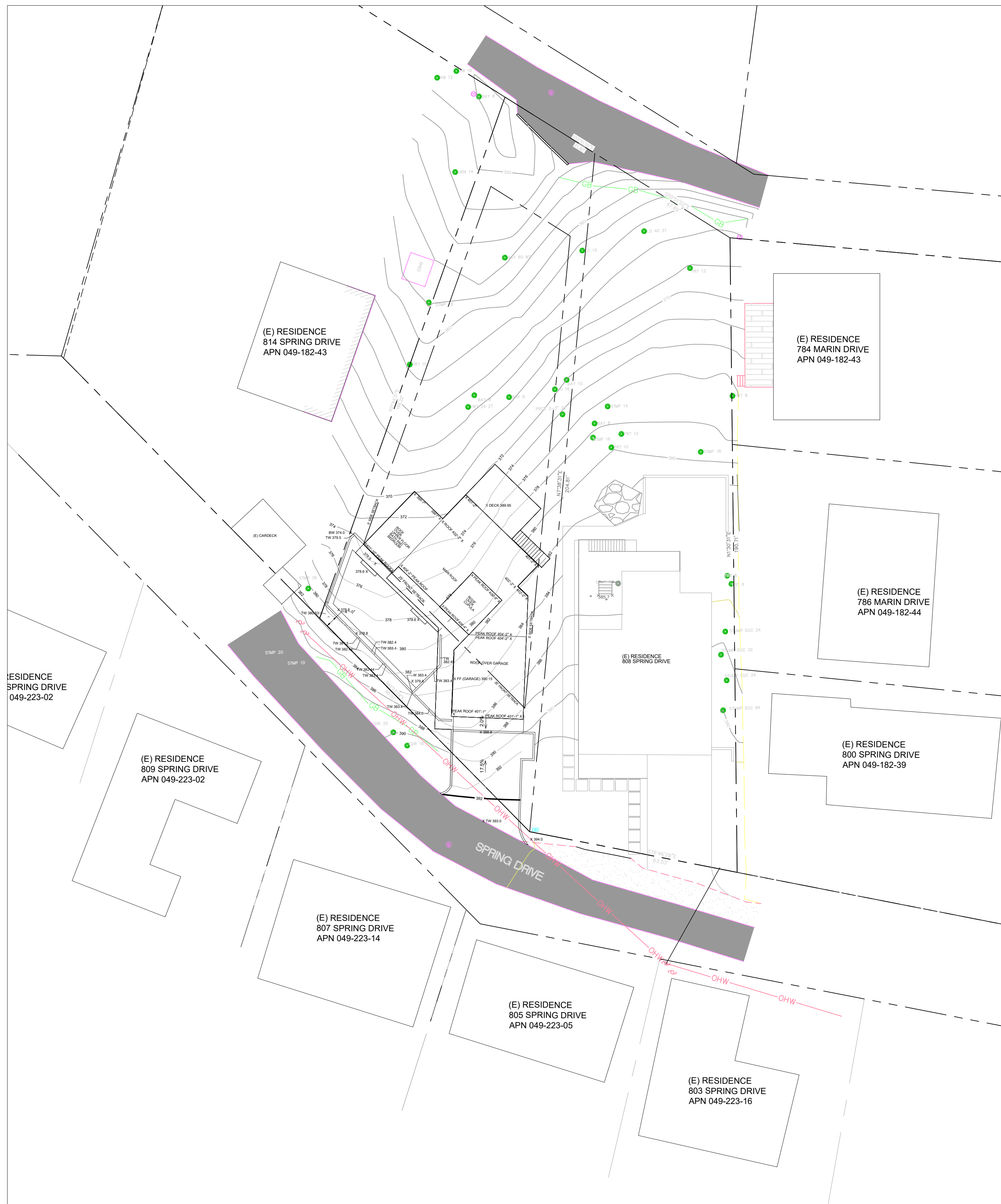
SITE PLAN W/ EXISTING COUNTOUR FOR BUILDING HEIGHT VERIFICATION SCALE 1" = 20'
