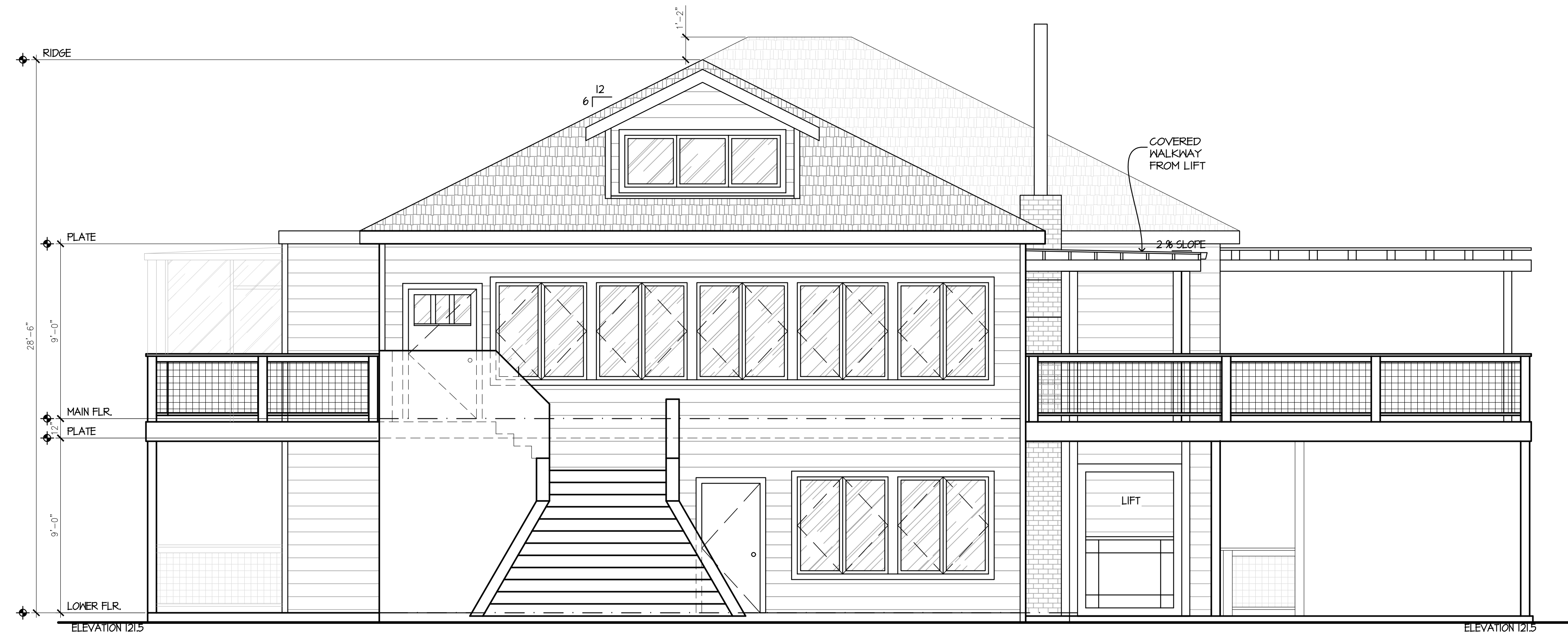
PROPOSED FRONT ELEVATION - NORTH Scale: 1/4" = 1'-0"
