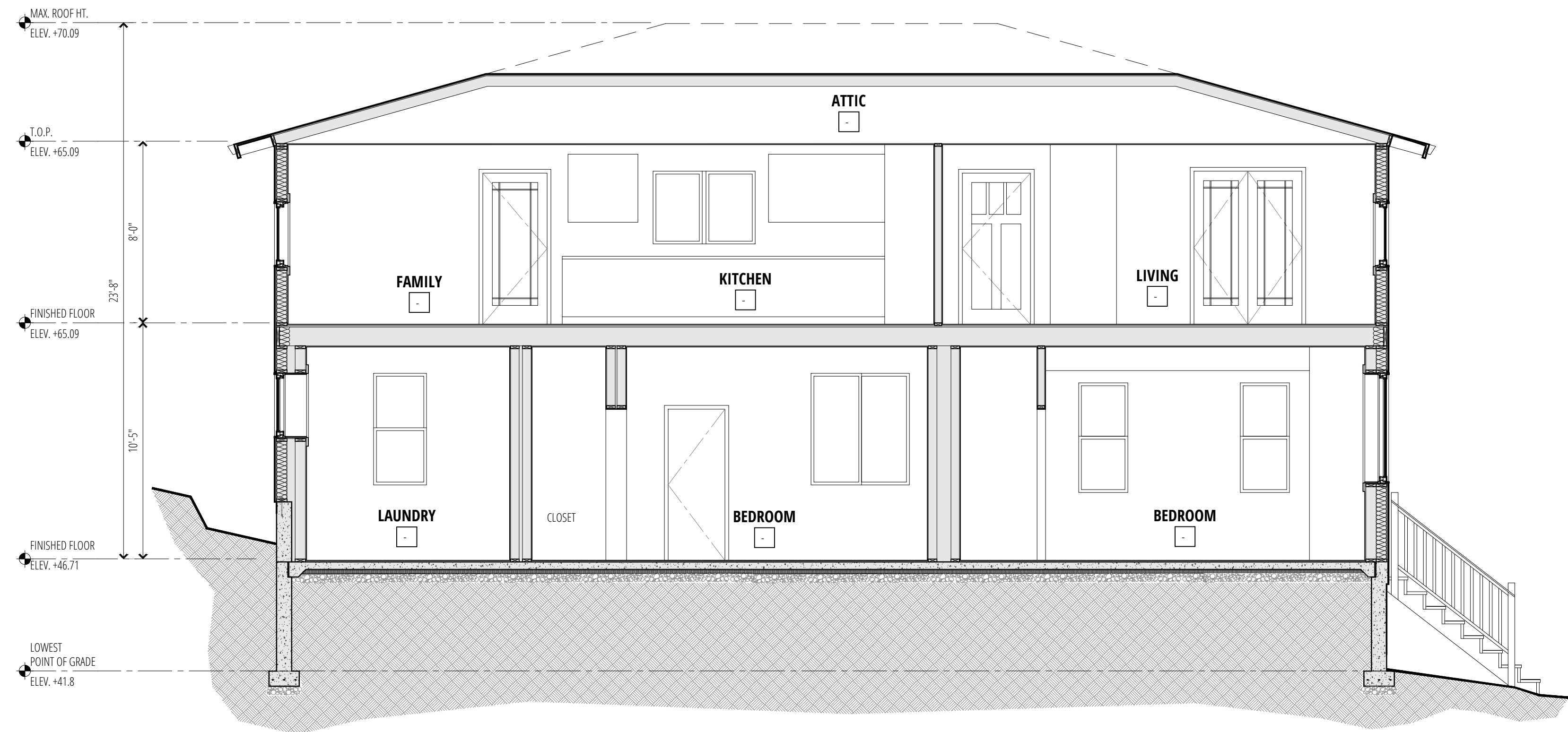
1 A4.0 EXISTING BUILDING SECTION SCALE: 1/4" = 1'-0"
