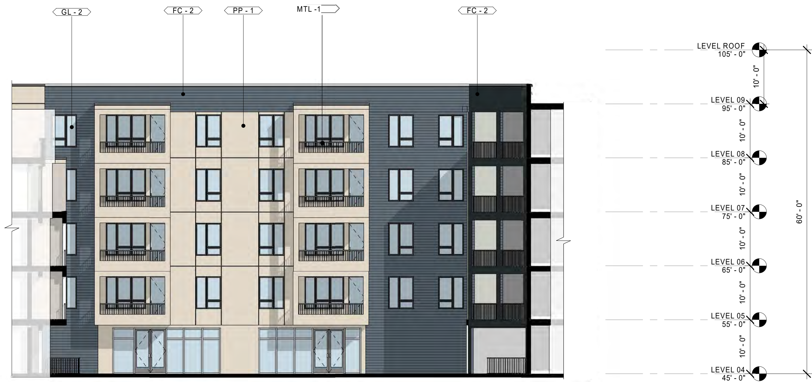
1 EHP BUILDING - COURTYARD NORTH ELEVATION 3/32" = 1'-0"
