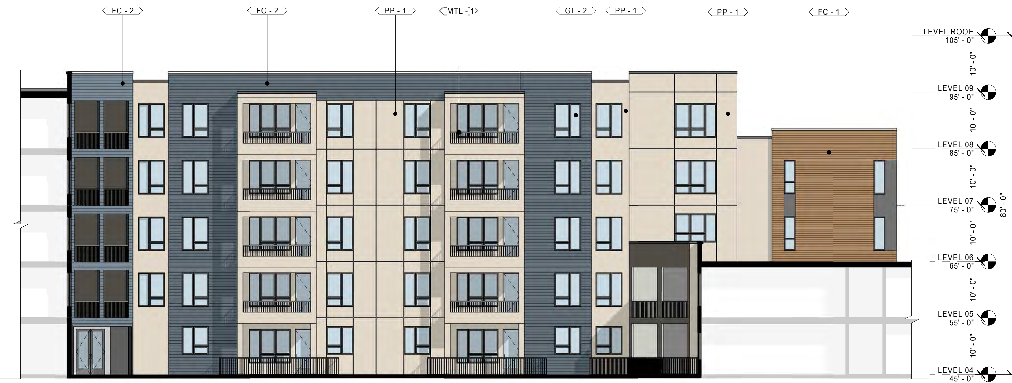
2 EHP BUILDING - COURTYARD EAST ELEVATION 3/32" = 1'-0"
