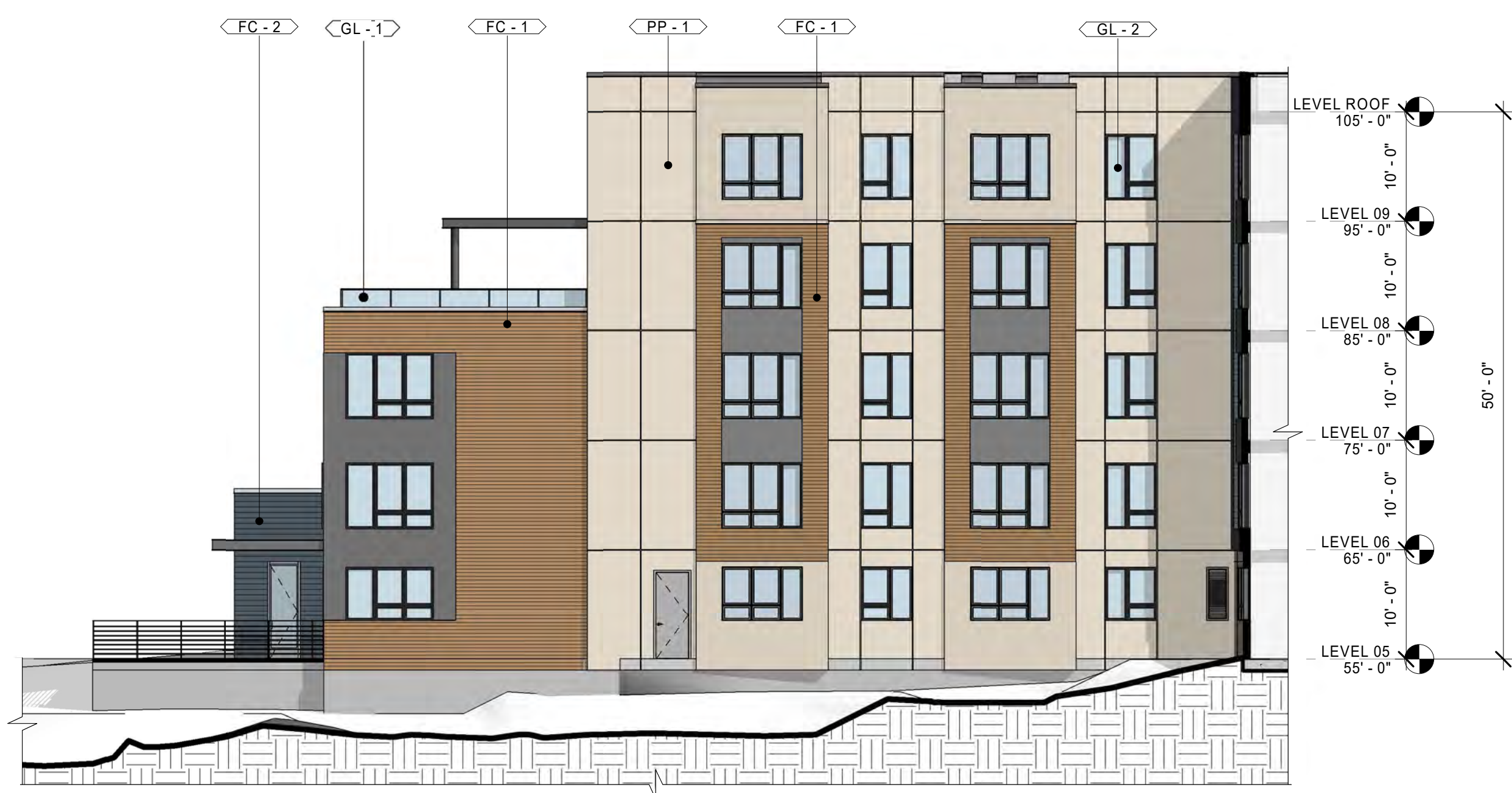
1 EDEN BUILDING - WEST ELEVATION LOBBY COURTYARD 3/32" = 1'-0"
