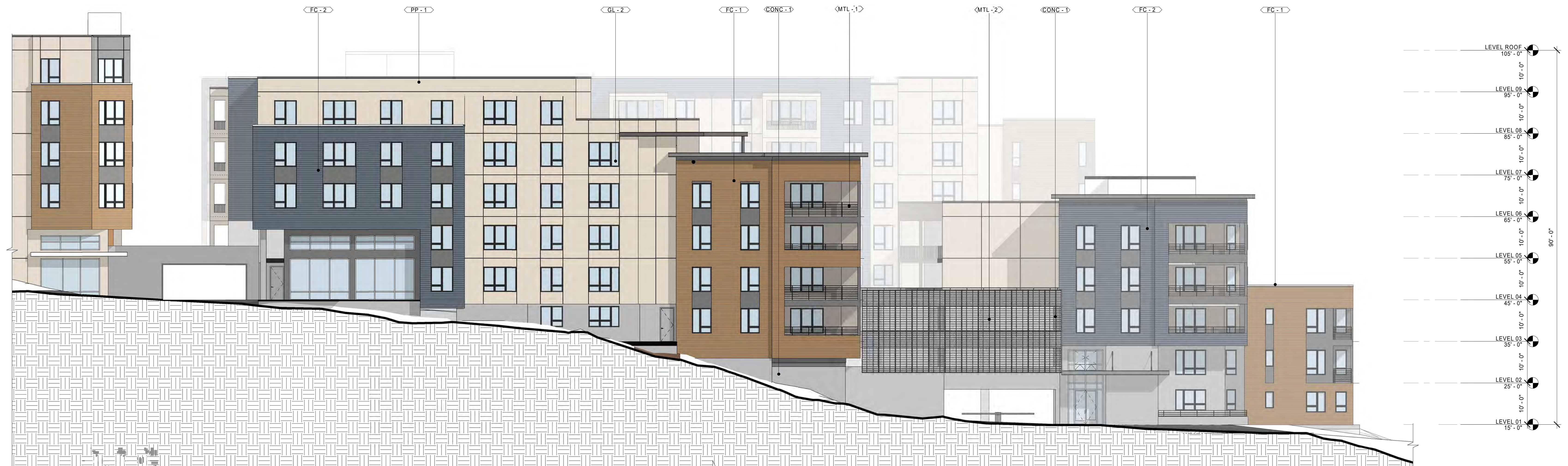
2 EHP BUILDING - WEST ELEVATION 3/32" = 1'-0"
