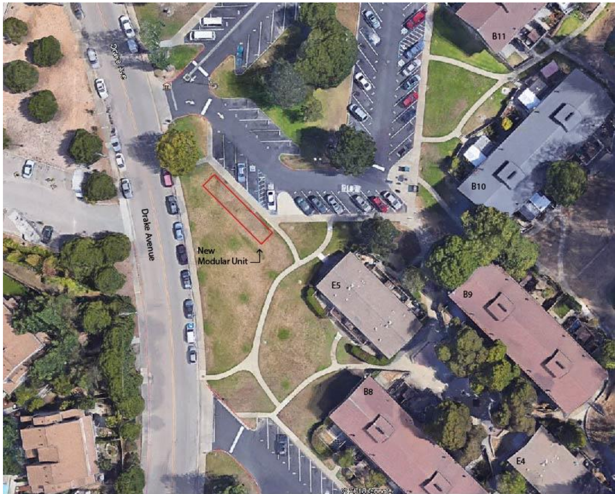
Figure 2: A site plan illustration of the proposed location and orientation of the 64' x 12' modular unit, shown in red. North is up, Highway 101 is to the east; not to scale. Courtesy: Google Earth, 2019
