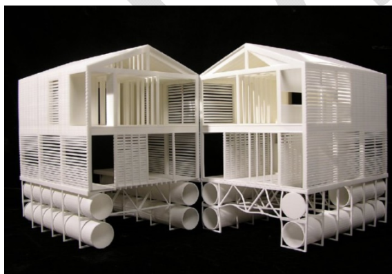
Home placed upon a steel pontoon flotation network (MOS Architects)
