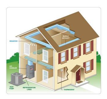
Using an air source heat pump system can reduce the amount of electricity you use for heating by 50 percent, compared to electric resistance heating such as furnaces and baseboard heaters.
