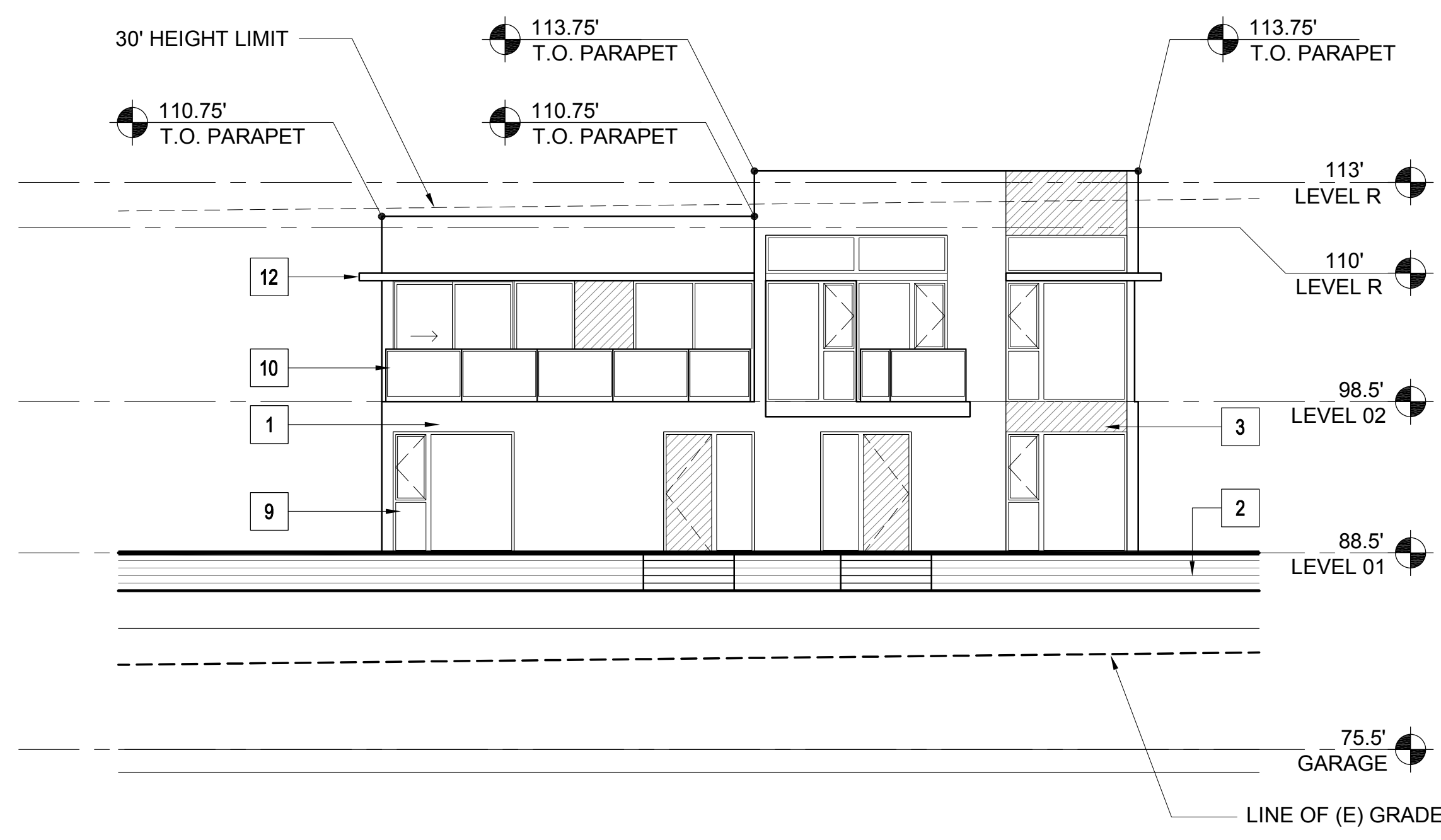
1 BUILDING 30.b- SOUTH ELEVATION 1/8" = 1'-0"
