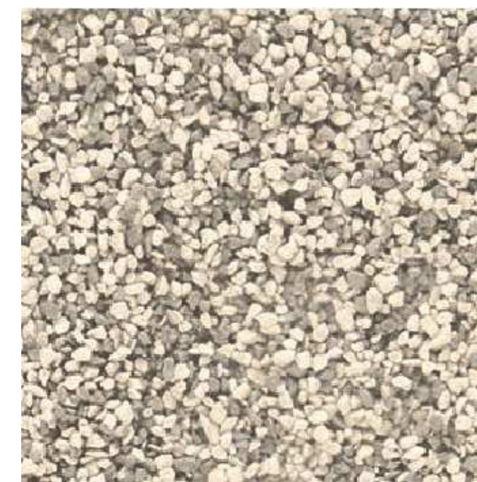
5B MEMBRANE ROOF (WITH BALLAST)
