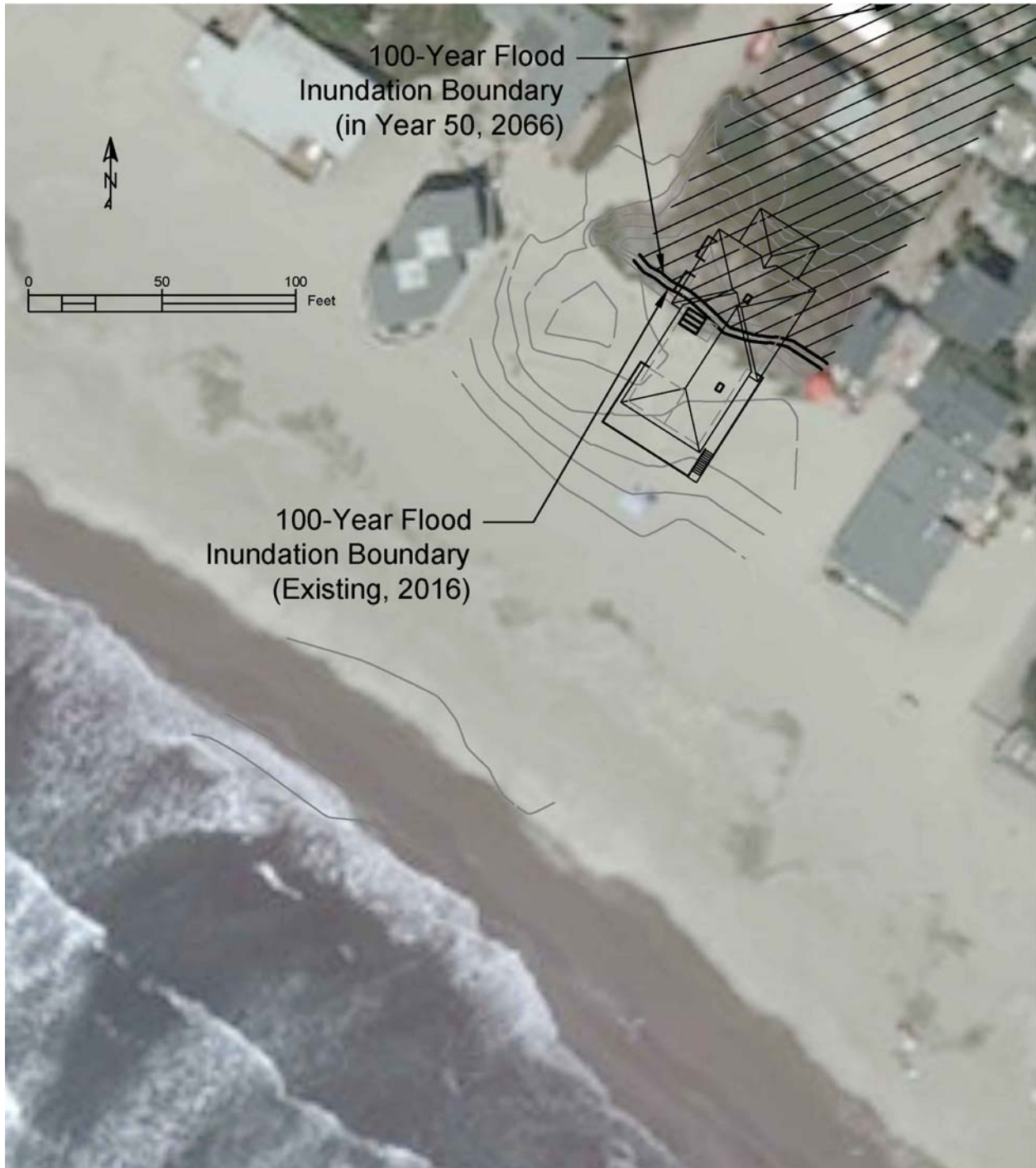
Figure 9. Existing and Future 100-Year Flood Inundation Boundaries
