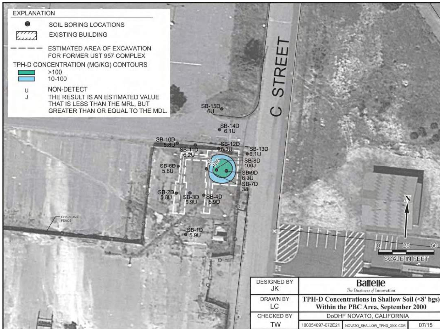
Figure 11. TPH-D Concentrations in Soil in the Former UST 957 Area (September 2000)
