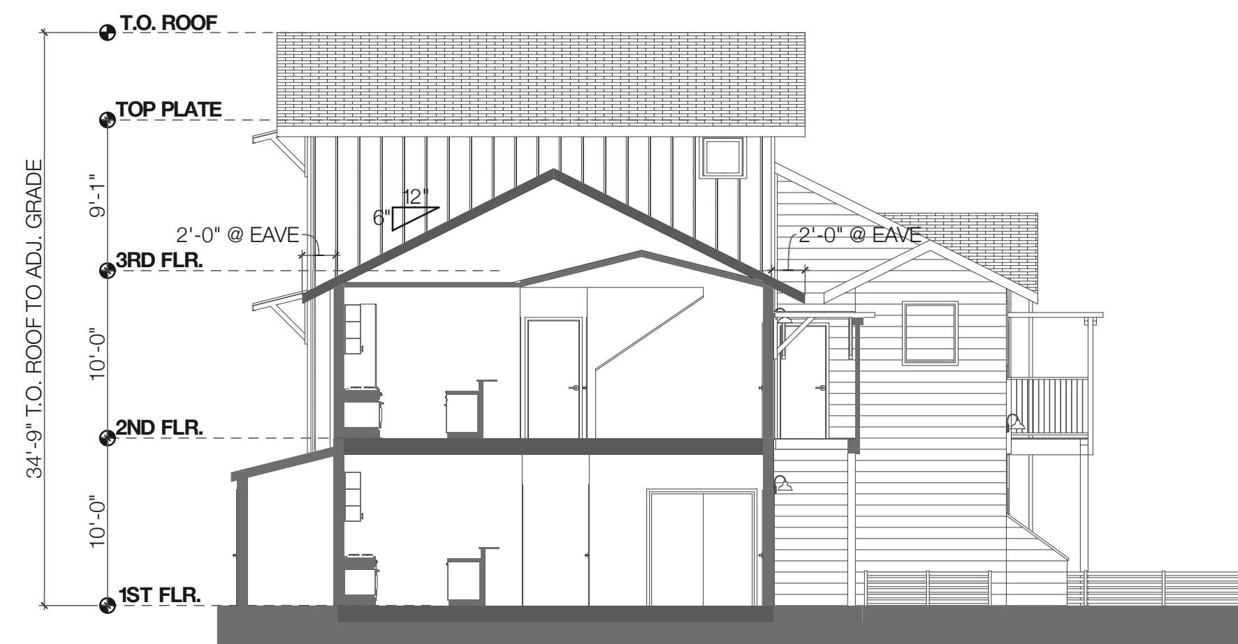
6 BUILDING SECTION SCALE: 1/8" = 1'-0"
