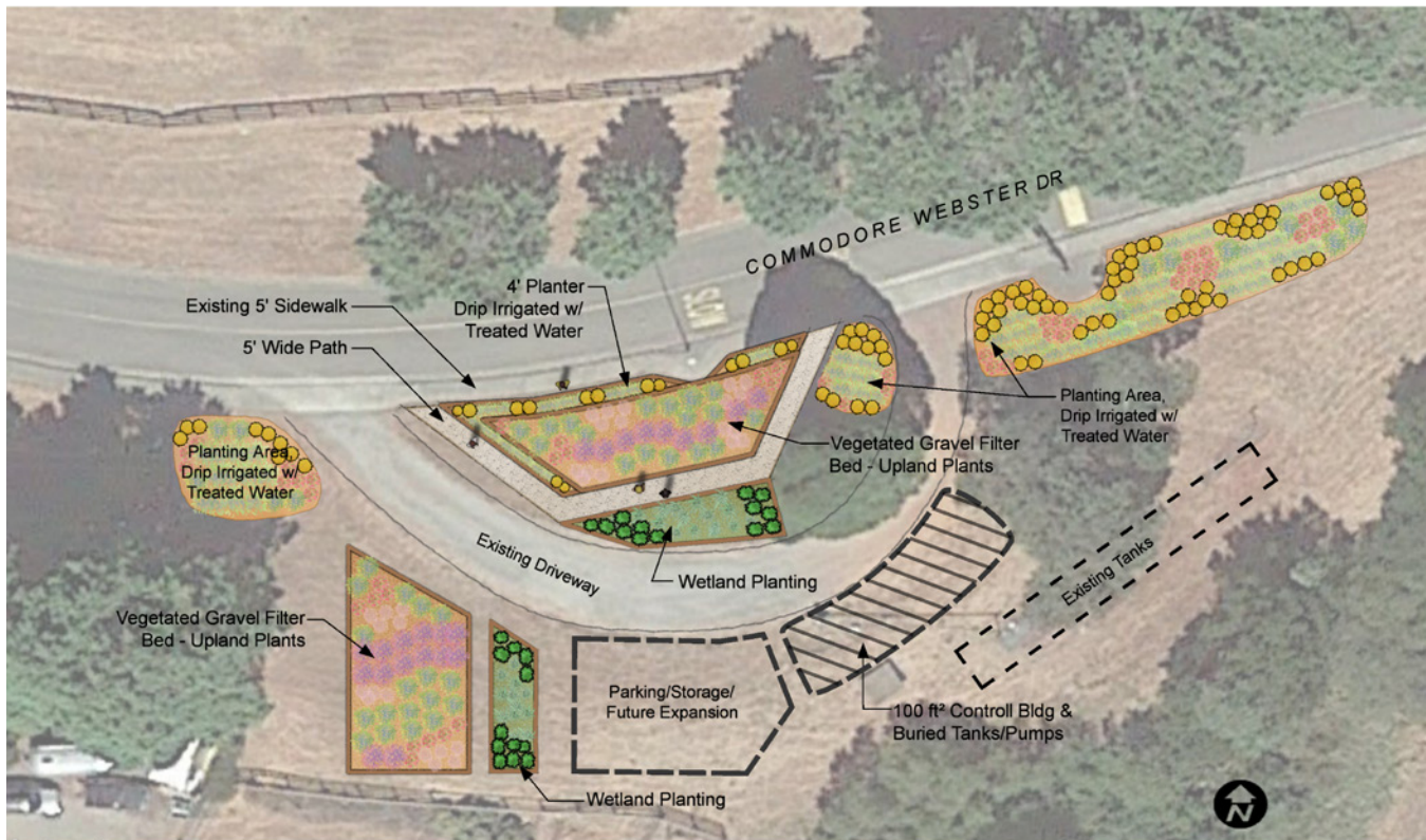
PLAN VIEW OF WASTEWATER TREATMENT SYSTEM
