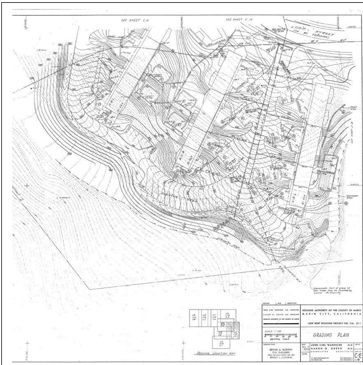
Figure 17. The 1958 civil plan set includes a grading plan for south side of site showing the service road and high-rise cluster. The plan shows how the steep topography was sensitively manipulated. Source: MHA onsite archives.
